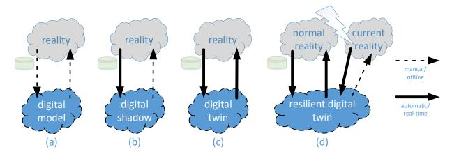
Figure 1: The difference between a digital model (a), a digital shadow (b), a digital twin (c), and a resilient digital twin confronted with a disruption (d). Visualization is based on (van der Aalst 2021a).
