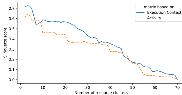
Fig. 6: Quality of discovery results measured by their silhouette scores, per selected number of clusters
