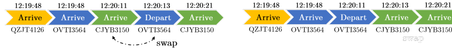
(a) Event data with sensor fault, where a package arrives on the next device before departing the previous device. (b) Repaired event data with sensor fault, where the timestamps of the implausible arrival and departure are swapped.
