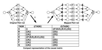
Fig. 2. Mapping of a PN with more than one place between two tasks (or transitions).
