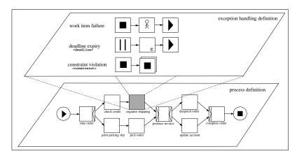
Fig. 3. Exception handling in relation to workflow processes
