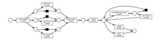
Fig. 7. The Petri net with the "time-out" transition made invisible.
