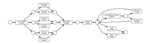
Fig. 3. The Petri net model resulting from applying the alpha algorithm on some event log.
