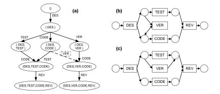
Fig. 2. Generated and Synthesis Approach: (a) Transition Systems (b),(c) Petri Nets
