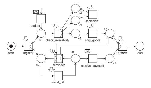
Figure 4: A WF-net modeling the handling of orders. The top part models the logistical part of the process while the bottom part models the financial part.
