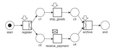
Figure 7: A superclass WF-net.
