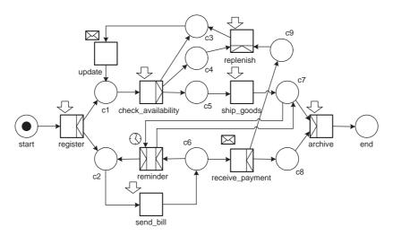
Figure 5: An incorrect WF-net. Place c9 has been added to model that a replenishment order can only be placed if the customer has paid. However, because of this addition the process can deadlock and a token is left behind in the process if no replenishments are needed.
