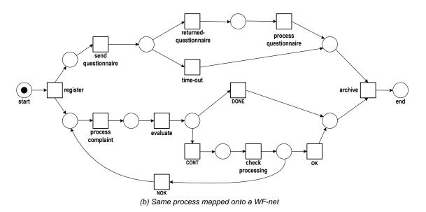
Fig. 1. A BPMN model and its corresponding WF-net. A WF-net is a Petri net with a start and an end place. The goal is that a case initiated via place *start* successfully completes by putting a token in place *end*.
