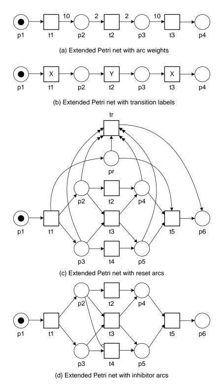
Fig. 3. Four extended Petri nets illustrating the different extensions.
