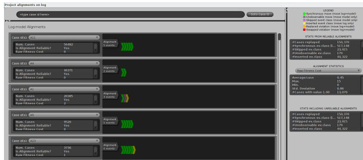
Figure 17: Example screen shot of conformance statistics projected onto cases in the event log.
