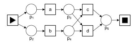
**Fig. 1.** Process model  $P_1 = \{(\{\triangleright\}, \{a\}), (\{\triangleright\}, \{b\}), (\{a\}, \{c, d\}), (\{b\}, \{c, d\}), (\{c, d\}, \{\blacksquare\})\}$  composed of five places discovered from event log  $L_1 = [\langle \triangleright, a, b, c, \blacksquare \rangle^{31}, \langle \triangleright, b, a, c, \blacksquare \rangle^{27}, \langle \triangleright, a, b, d, \blacksquare \rangle^{23}, \langle \triangleright, b, a, d, \blacksquare \rangle^{19}]$ .
